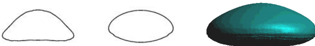
Figure 2.8: Simulation results of a bubble with a diameter of 6 mm. Left: CSF model; middle: tensile force model; right: 3D front tracking.
