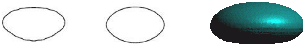
Figure 2.7: Simulation results of a bubble with a diameter of 4 mm. Left: CSF model; middle: tensile force model; right: 3D front tracking.
